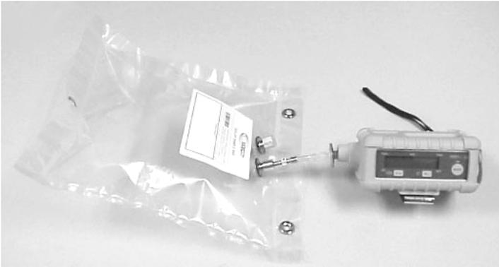
Figure 4-1 Connection of Calibration Gas
