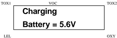
3. The LED should be red in color when charging. If the battery is fully charged, the LED will change from red to green. The red color indicates that the battery is being charged. The green color indicates that the battery is fully charged. The display will also indicate "Fully charged." A completely discharged MultiRAE PLUS monitor will be charged to full capacity within 10 hours.
