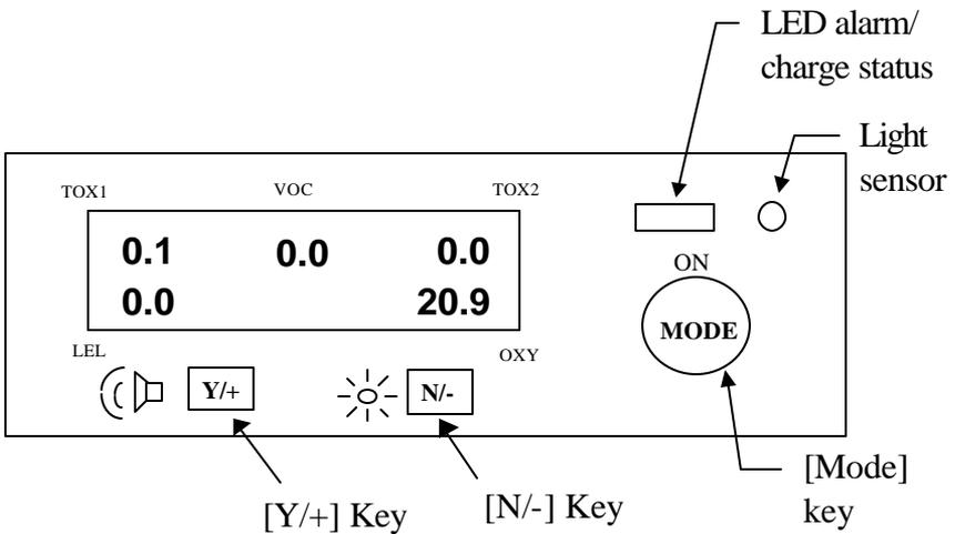
Figure 2-2 Key-pad and Display of the MultiRAE PLUS Multi-gas Monitor
