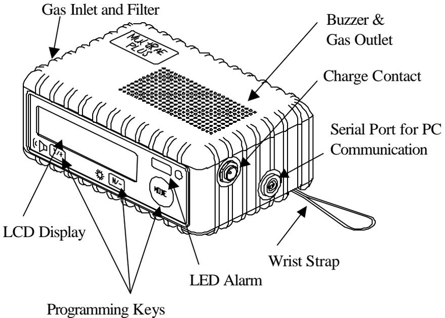
Figure 2-1 Major parts of the MultiRAE PLUS Multi-gas Monitor
