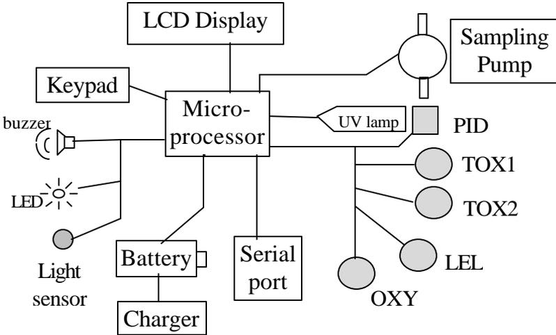
Figure 6-1 Block Diagram of MultiRAE PLUS Monitor
