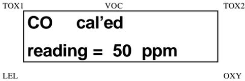
If no gas has reached the sensor after 60 seconds, the display will show "No gas flow..." and abort the calibration.
