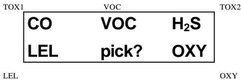
2. Turn on the valve of the CO gas bottle to start the flow of the span gas. Display shows “Apply CO Gas” and will wait for the calibration gas to reach the sensor. When the calibration gas has reached the sensor the display will show “calibration in progress...60” with the countdown timer shows the number of remaining
